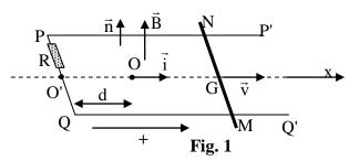
At an instant t, G has an abscissa  $\overline{OG} = x$  and a velocity  $\vec{v}$  of algebraic value v (Fig. 1).
