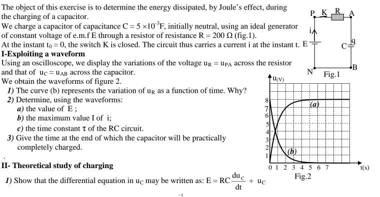
2) The solution of this equation has the form  $u_C = A e^{\frac{-t}{\tau}} + B$  where A, B and  $\tau$  are constants.
