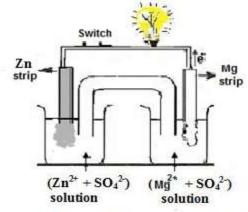
Schema of functioning galvanic cell G1
